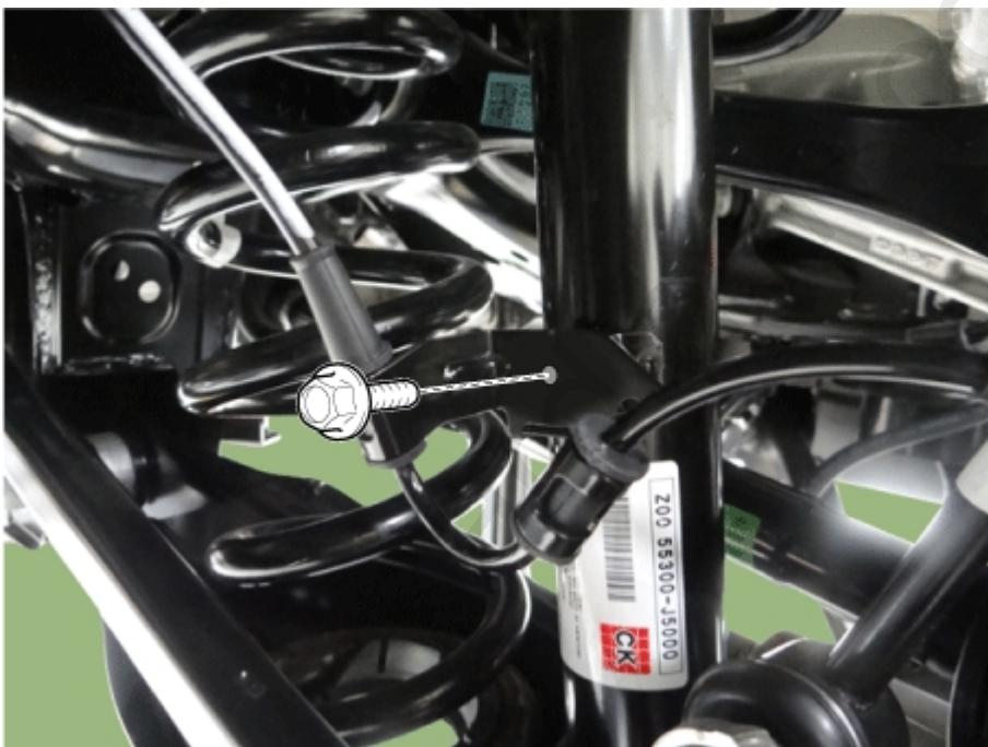
4. Disconnect the rear wheel speed sensor connector.
